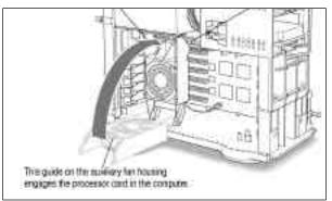
Lifting the auxiliary fan (retaining clip on 8500)
